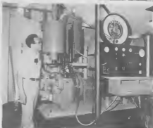
Max Fingal of the Labs with one of the units which determine knock characteristics of gasoline products.
